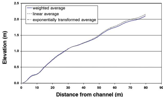
**Figure 5. Representative slope profiles using three different methods to represent slope values from multiple flowpaths for the top hillslope profile of Watkinsville watershed P2.**
