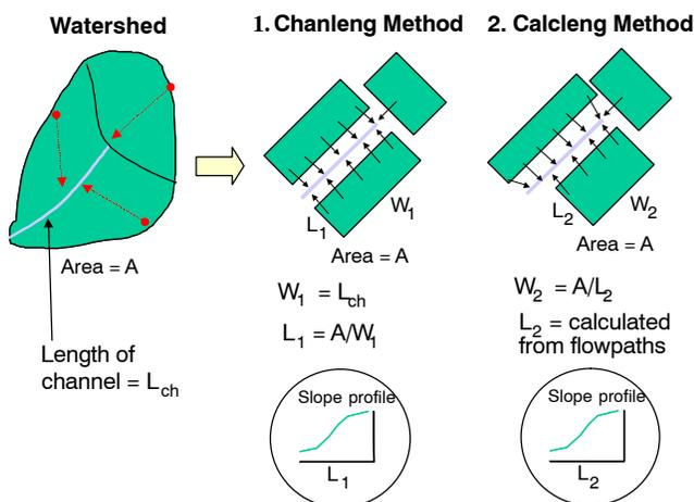
Figure 4. The Chanleng and Calcleng methods for watershed discretization.
