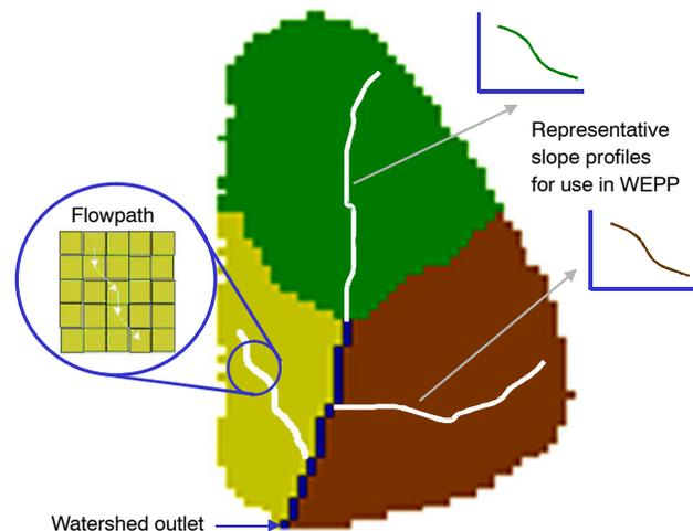
Figure 3. Flowpaths in watershed modeling derived from grid-based DEMs.
